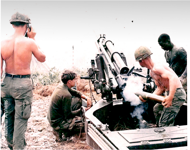
Artillerymen of Battery C, 1st Battalion, 21st Artillery, 1st Cavalry Division (Airmobile), load a round into a 105-mm. howitzer.
