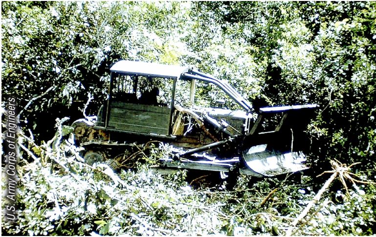
A modified D7E bulldozer equipped with a Rome plow and an armored cab
